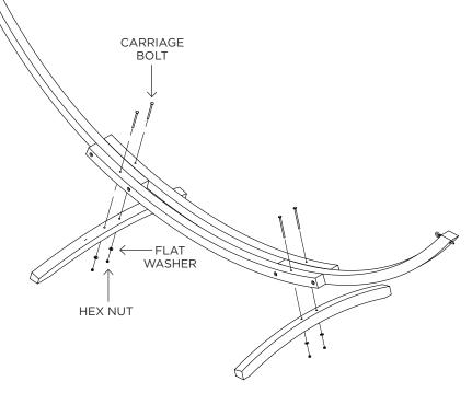
in each foot with the holes in the center beams. The slant on the base of the foot should angle the foot in towards the center of the stand. Insert (4) carriage bolts, (4) flat washers, and (4) hex nuts like shown in the diagram. **Tighten all bolts**.
